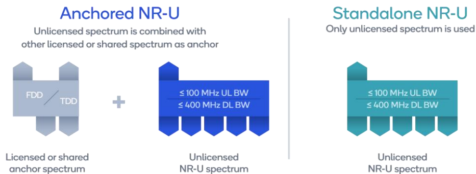
Figure 2: 3GPP Release 16 on 5G NR-U, Source: Qualcomm
