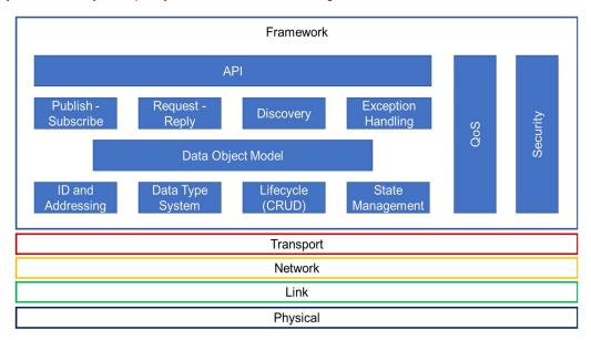
Figure 5. Connectivity in framework layer functions
