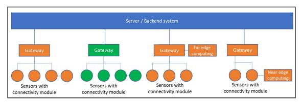
Figure 3. Multiple connectivity types with multiple gateways
