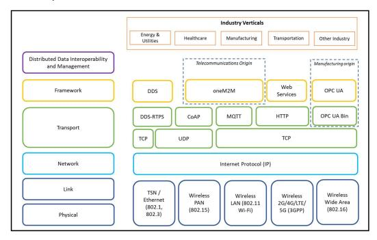
Figure 7. IIoT connectivity framework
