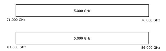
4.2 In order to provide high capacity link via FDD or TDD technique, issuance of an assignment will be based on a single channelling plan of 5.000 GHz bandwidth. The issuance of an assignment shall be made based on the channelling plan in **Appendix B.**
