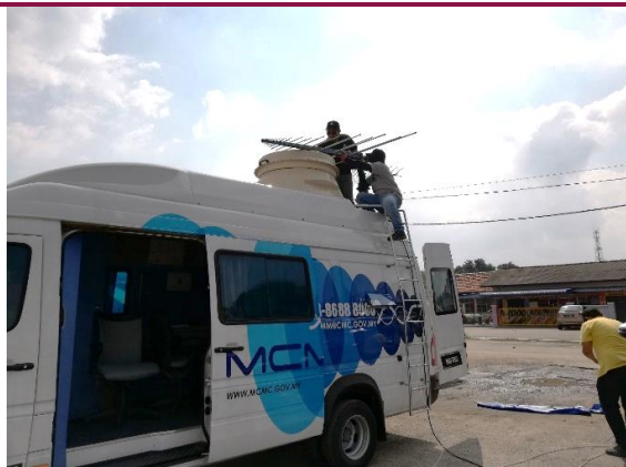
Figure 5.33 Antennas for DTT Signal Measurement
